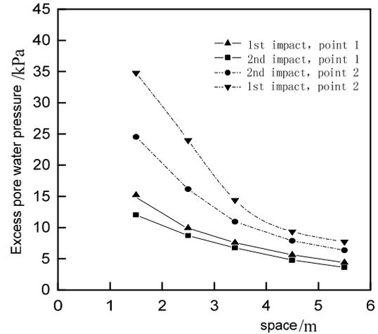
Fig 3.7 Variation of the peak value of excess pore water pressure with horizontal distance
