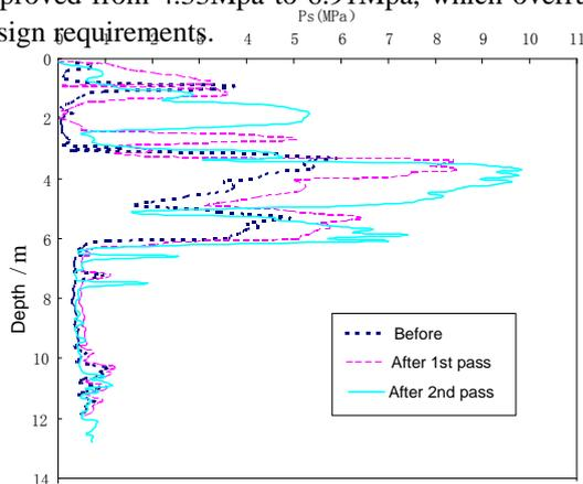
Fig 3.9 CPT test results between before and after soil improvement
