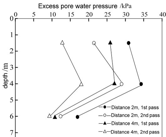
Fig 3.6 Variation of the increment of excess pore water pressure with the impact number
