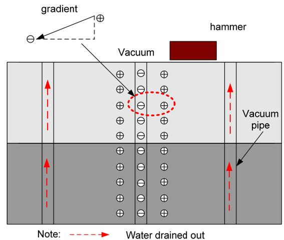
Fig 2.1 the primary mechanic of HVDM method
