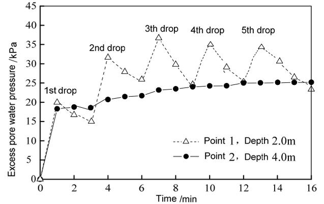
Fig. 3.3 The increasing curves of excess pore water pressure of single point impact
