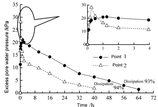
Fig 3.5 Dissipation curves of excess pore water pressure of single point impact (2<sup>nd</sup> pass)
