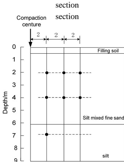
Fig 3.2 Arrangement of the pore water pressure gauges in the location of single point impact
