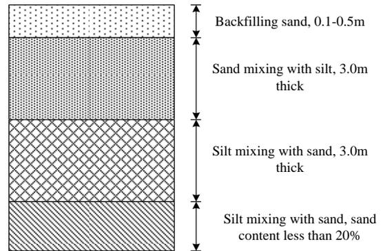
Fig 3.1 soil condition section
