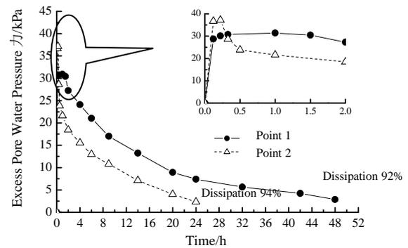
Fig 3.4 Dissipation curves of excess pore water pressure of single point impact (1<sup>st</sup> pass)
