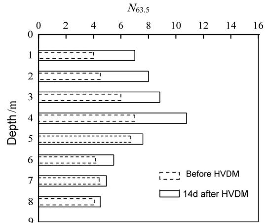
Fig.3.10 SPT test results between before and after soil improvement
