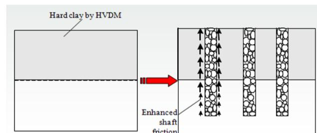
Figure 3. HVDM plus stone columns as composite foundation.
