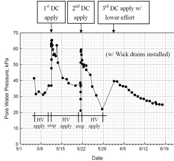
Figure 8. Pore pressure response due to PVDs and vacuum dewatering.
